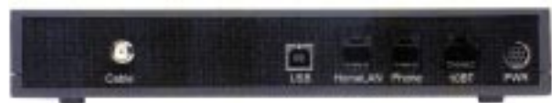
This Zoom cable modem for the US shows the sort of device that may come with an open market in fast links. It has built-in ports for USB, Ethernet or phone-net links and an 802.11 wireless net slot. Curiously, there is no 1394 link.
